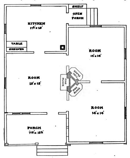
FIG. 64.—PLAN OF TYPICAL SOUTHERN COTTON-MILL FRAME COTTAGE.
